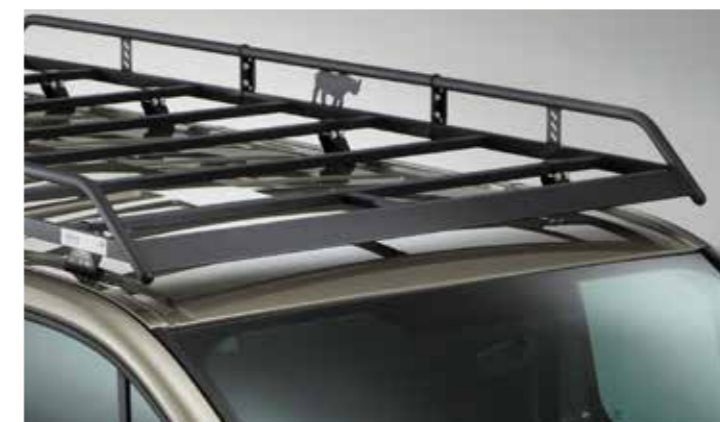
Aerofoil reduces overall wind noise and drag
